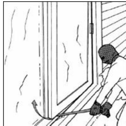
Figure 2 Rotating motion of the panel caused by prying action, can break the lock.
